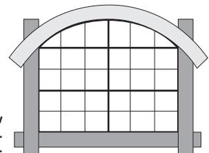
For arched window follow above instructions but allow extra length to accommodate radius of window. Use Window Tape 25 mil for sill and jamb flashing.
